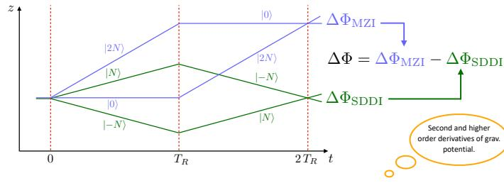
The differential phase of this AlF is especially sensitive to **gravitational curvature**.
